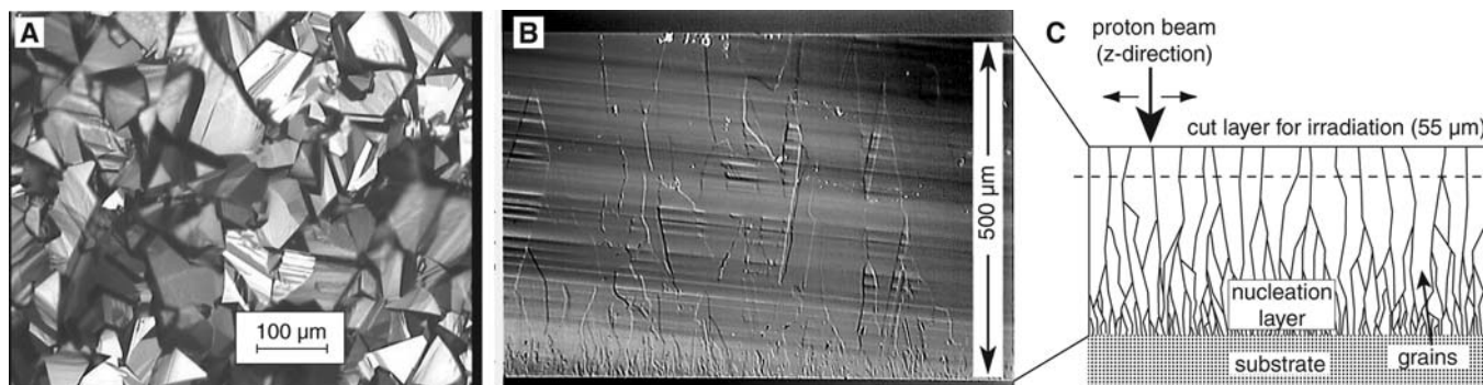
Fig. 2. (A) Surface view of the unpolished polycrystalline CVD diamond sample. (B) Cross-sectional image of the original 500- \mu\text{m} -thick polished sample, showing the columnar structure of the diamond layer. Grain sizes increase with distance from the nucleation layer to about 50 \mu\text{m} wide
